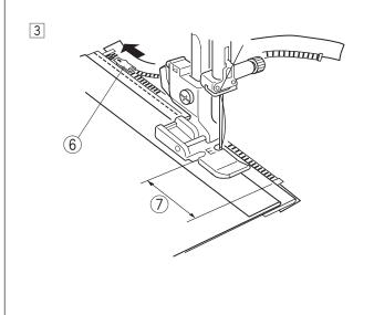
3 Sew through all layers next to the fold. Stop the machine 5 cm (2") before the foot reaches the slider on the zipper tape.
