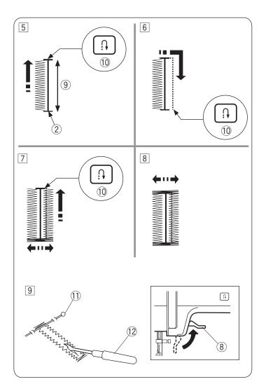
5 Sew the left side up to the required length of the buttonhole.
