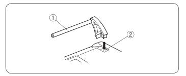
Setting the Spool Pin Insert the spool pin into the hole as shown.
