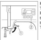
Raise the presser foot lifter. Turn the power switch ON. Press the needle up/down button to raise the thread take-up lever to its highest position.
