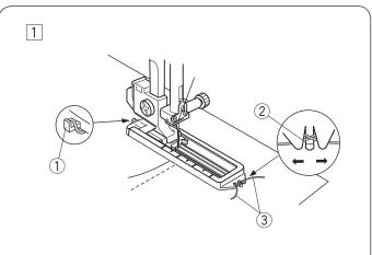
Use the same procedure as the memory buttonhole sewing (refer to pages 28-29). Set the stitch width to match the thickness of the cord used.
