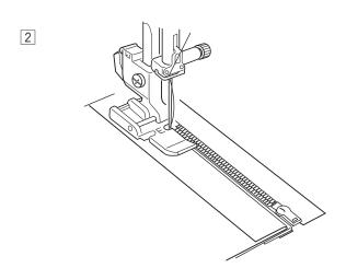
2 Attach the zipper foot E with the pin on the right hand
