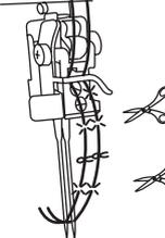
**4** Before starting sewing, clear the needle threads from under the presser foot to make sure they are not caught below the needle plate. Draw the needle threads in the direction A. Then pull out the threads to the back approximately 10 cm (4") away from the presser foot. Lower the presser foot, and you are now ready to sew.
